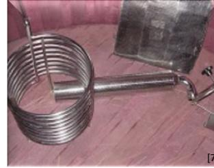
The basis is similar to that of the cooling jackets but, in this technique, cold is transferred by introducing plates or coils into the tank coming into contact with the product (must).
