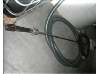
It is based on the application of direct heat to the liquid inside the tank, controlling the temperature with a digital thermostat to avoid any evaporation of scents. It is generally used for the malolactic fermentation or excessively cold areas.
