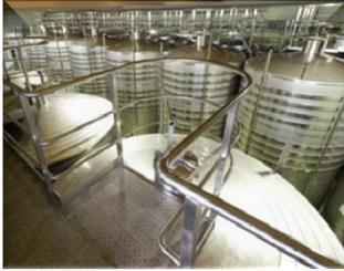
Jackets surrounding the tanks allow the transmission of heat or cold by means of a fluid circulating inside them.
