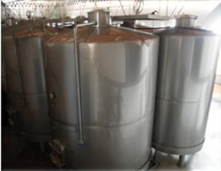
In this technique, water is sprayed into the outside part of the tanks in order to reduce the inner temperature.
